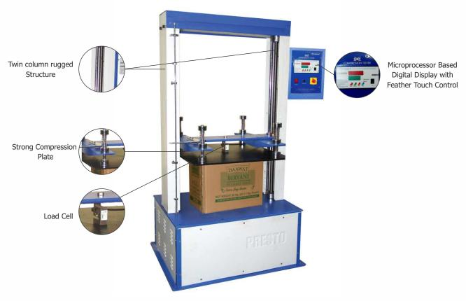
**Box Compression Tester Digital** is a consistent tool to indicate the Compression strength of cardboard boxes so that it does not get deformed or crushed when stacked one above the other during storage or transit. PRESTO Box Compression Tester is manufactured under various Test Standards ASTM D642, ASTM D4169, TAPPI T804, ISO 12048, and JIS Z0212. Available in Computerized model also.
