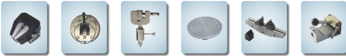
Self Tighting grip Wedge Type grip Vice Type grip Compression Plate Flexural Roller Type Grip
